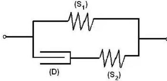
Figure 3.3: A diagram of a Standard Linear element
