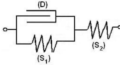
Figure 3.4: A diagram of a Standard Solid element
