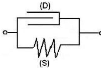
Figure 3.2: A diagram of Kelvin-Voigt element
